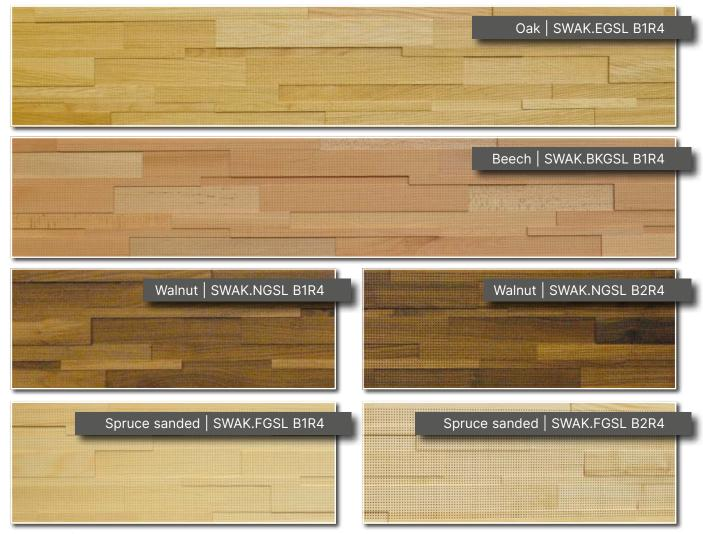
STEPWOOD $^{\circ}$  Acoustic Panels are L 1250 x W 219 mm and are grooved all around. The surface is always sanded and painted. Backed with acoustic fleece in black. The absorption value is determined by the construction height and the insulating material. For all further technical details see page 22.
