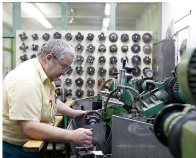
Each profile has its own tool manufactured and serviced in our workshop.
