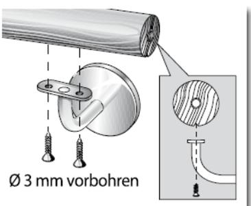
Screw the handrail support with the support in the **groove** of the handrail. (Countersunk screw 3.5x25 mm)
